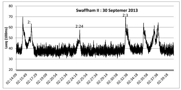
3.32 There was significant amplitude modulation of the turbine noise signal as can be seen in the trace below and other samples at Appendix 2.
